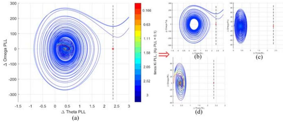
Fig. 12. Phase portrait for scenario-2: decreasing  $K_{ipll}$  (blue to red). (a) 3 to 0.16 times  $K_{ipll}$ . (b) Stage-1: 3 to 2.82 times  $K_{ipll}$ . (c) Stage-2: 2.69 to 2.50 times  $K_{ipll}$ , and (d) Stage-3: 2.44 to 0.16 times  $K_{ipll}$ .
