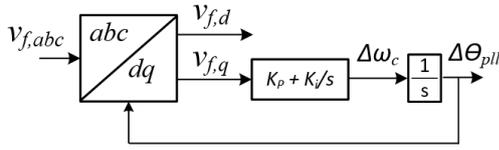
Fig. 2. Block diagram of the SRF-PLL.
