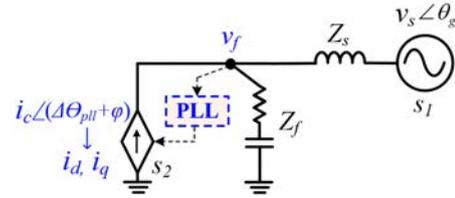
Fig. 3. Reduced order VSC-grid system for stability analysis.
