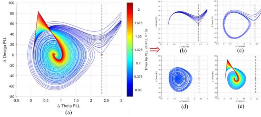
Fig. 9. Phase portrait for scenario-1: increasing  $Kp_{pll}$  (blue to red). (a) 0.05 to 2 times  $Kp_{pll}$ , (b) Stage-1: 0.05 to 0.26 times  $Kp_{pll}$ , (c) Stage-2: 0.28 to 0.36 times  $Kp_{pll}$ , (d) Stage-3: 0.38 to 0.50 times  $Kp_{pll}$ , and (e) Stage-4: 0.52 to 2 times  $Kp_{pll}$ .
