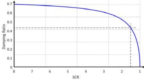
Fig. 6. Damping ratio of reduced VSC-grid model versus SCR,  $K_{ppll} = 0.1$  and  $K_{ipll} = 10$ . Optimal damping at SCR = 8.
