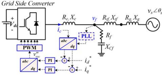
Fig. 1. Single-line diagram of a grid-connected VSC using the typical vector current control.
