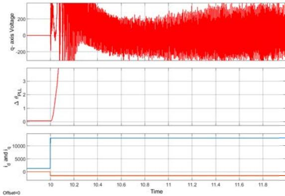
Fig. 13. Results from detailed simulation model. First swing angle instability in scenario-1 (SCR=3) with 0.05 times  $K_{ppll}$ .
