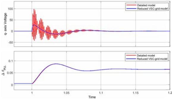
Fig. 7. Detailed simulation model vs Reduced order analytical model: q-axis filter bus voltage and the angle tracked by the PLL.
