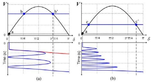
Fig. 8. Unstable PLL synchronisation scenario: (a) higher operating point, (b) lower operating point. Instability classified as 1st or multi swing instability.
