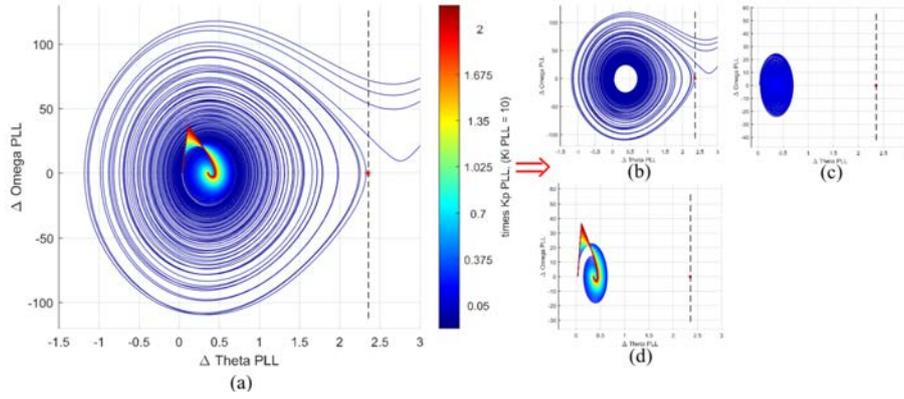
Fig. 11. Phase portrait for scenario-2: increasing  $K_{ppll}$  (blue to red). (a) 0.05 to 2 times  $K_{ppll}$ . (b) Stage-1: 0.05 to 0.11 times  $K_{ppll}$ . (c) Stage-2: 0.13 to 0.30 times  $K_{ppll}$ , and (d) Stage-3: 0.32 to 2 times  $K_{ppll}$ .
