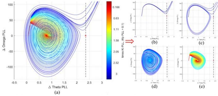
Fig. 10. Phase portrait for scenario-1: decreasing  $Ki_{pll}$  (blue to red). (a) 3 to 0.16 times  $Ki_{pll}$ , (b) Stage-1: 3 to 2.88 times  $Ki_{pll}$ , (c) Stage-2: 2.83 to 2.69 times  $Ki_{pll}$ , (d) Stage-3: 2.64 to 2 times  $Ki_{pll}$ , and (e) Stage-4: 1.9 to 0.16 times  $Ki_{pll}$ .
