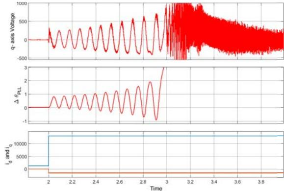
Fig. 14. Results from detailed simulation model. Multi swing angle instability in scenario-2 (SCR=1.2) with 0.2 times  $K_{ppll}$ .
