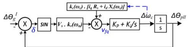
Fig. 4. Equivalent diagram of the reduced VSC-grid model.
