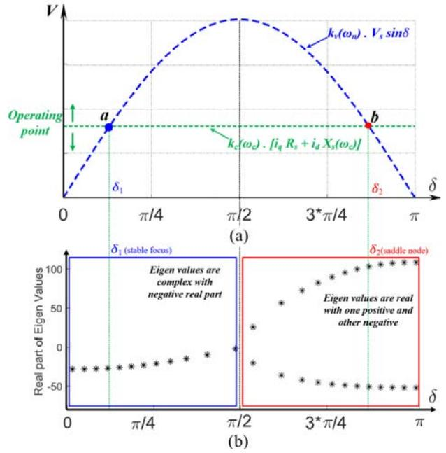
Fig. 5. (a) Existence of equilibrium points, (b) Eigenvalue analysis with varying grid impedance. Equilibrium point 'a' is a stable focus, i.e. stable point. Whereas, the equilibrium point 'b' is a saddle node, i.e. unstable point.
