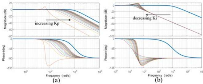
Fig. 15. Bode plots: (a) increasing  $K_{p_{pll}}$ , (b) decreasing  $K_{i_{pll}}$ . Bold blue line represents a illustrative current controller bode plot.
