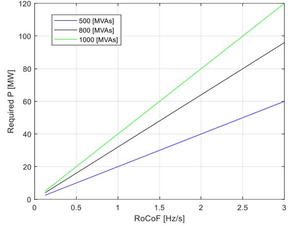
Figure 12: Required active power versus maximum ROCOF for different equivalent inertias.
