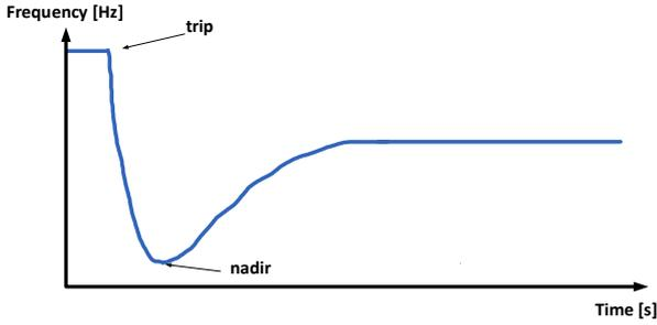
Figure 11: Frequency containment process (under-frequency case).
