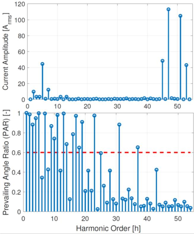
Fig. 4: Current harmonic spectrum for WT 1 (M1) (top) and the respective PAR (bottom) for 1-min period when the carrier signal synchronization feature is enabled
