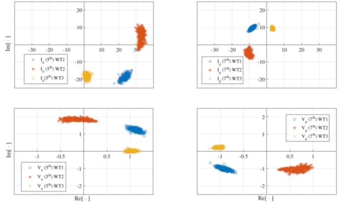
Fig. 8: Phasor diagram of the 5<sup>th</sup> and 7<sup>th</sup> harmonic order, current and voltage based on the sequence domain (SD) harmonic model during the operating points shown in Figure 3.
