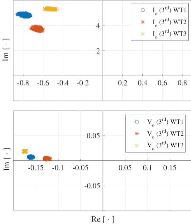
Fig. 7: Phasor diagram of the 3<sup>rd</sup> harmonic order, current and voltage based on the sequence domain (SD) harmonic model during the operating points shown in Figure 3.
