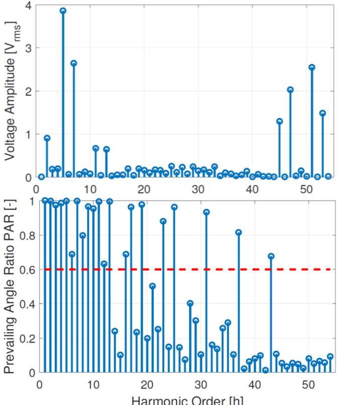
Fig. 5: Voltage harmonic spectrum for WT 1 (M1) (top) and PAR (bottom) for 1-min period when the carrier signal synchronization feature is enabled.
