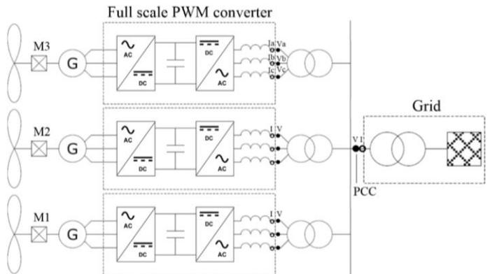
Fig. 2: AHOWPP installed measurement point locations.
