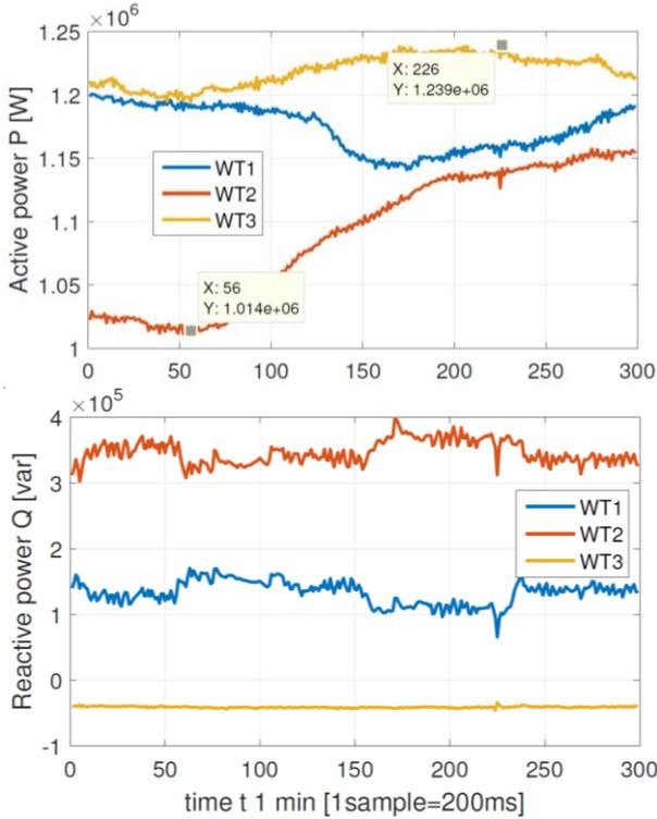
Fig. 3: The reactive power injection for all three WTs during 1 minute of operation, when PWM synchronizations feature is enabled and the active power operating point is approximately 30%.
