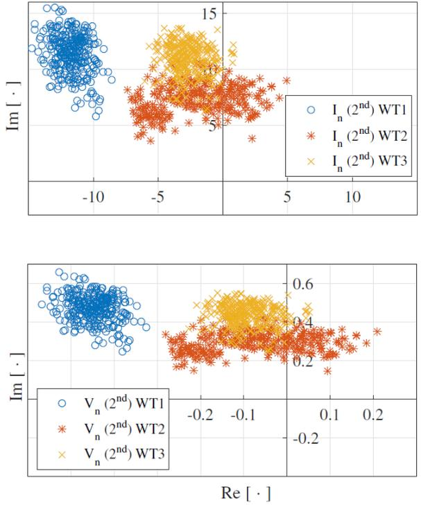
Fig. 6: Phasor diagram of the 2<sup>nd</sup> harmonic order, current and voltage based on the sequence domain (SD) harmonic model during the operating points shown in Figure 3.
