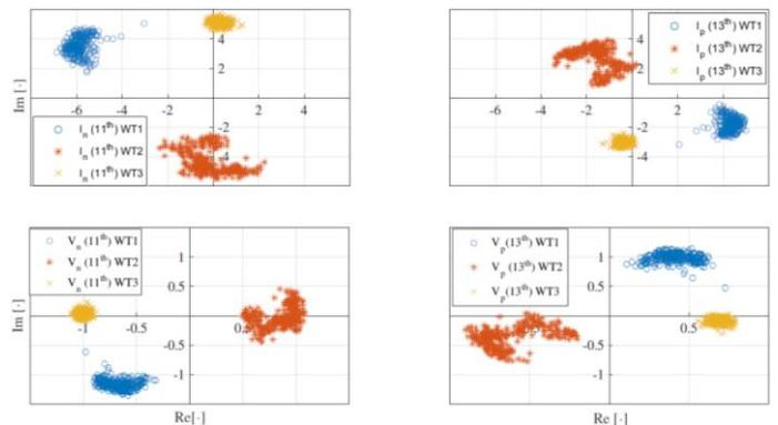
Fig. 9: Phasor diagram of the 11<sup>th</sup> and 13<sup>th</sup> harmonic order, current and voltage based on the sequence domain (SD) harmonic model during the operating points shown in Figure 3.
