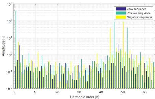
Fig. 10: Harmonic voltages spectrum in sequence component form at WT3 converter-side.
