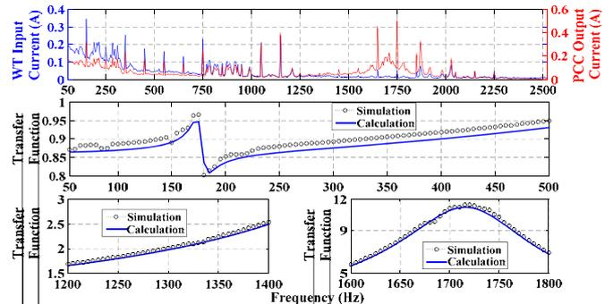
Fig. 12. PE from WT1 to grid. Upper figure: Input (left vertical scale) and output current spectrum at PCC (right vertical scale). Middle and bottom figures: TF obtained from simulations (ratio of output and input currents) and circuit model.
