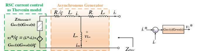
Fig. 4. Average model and single-phase controller model of RSC with AG based on [22, 23].
