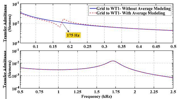
Fig. 11. SE TA from the grid to WT1 with and without converter average modelling. Upper figure: 0-0.5 kHz; lower figure: 0.5-2.5 kHz.
