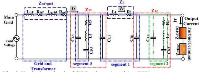
Fig. 8. Equivalent circuit of SE TA from the grid to WT1.
