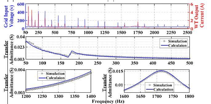
Fig. 13. SE from grid to WT1. Upper figure: Input voltage spectrum (left vertical scale) and output current spectrum at WT terminal (right vertical scale). Middle and bottom figures: TA obtained from simulations (ratio of output current and input voltage) and circuit model.
