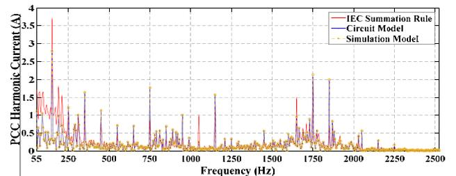
Fig. 14. Total PE at PCC obtained from circuit, simulation and IEC models.
