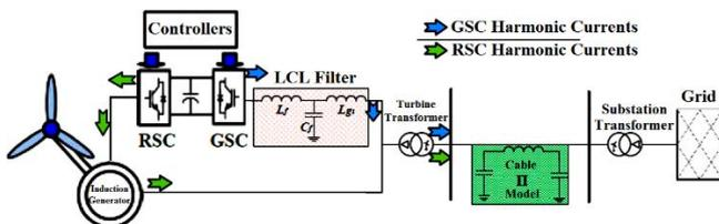
Fig. 2. Single-line diagram of a type III grid-connected WT.
