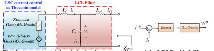
Fig. 3. Average model and single-phase controller model of GSC with LCL filter based on [22, 23].
