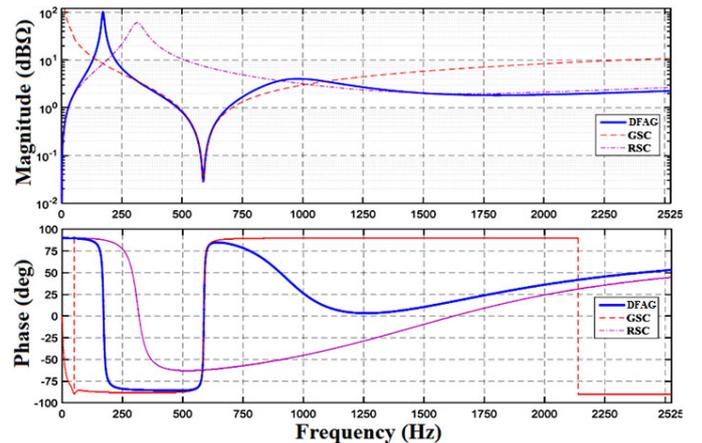
Fig. 9. Magnitude and phase of DFAG, GSC, and RSC output impedance.
