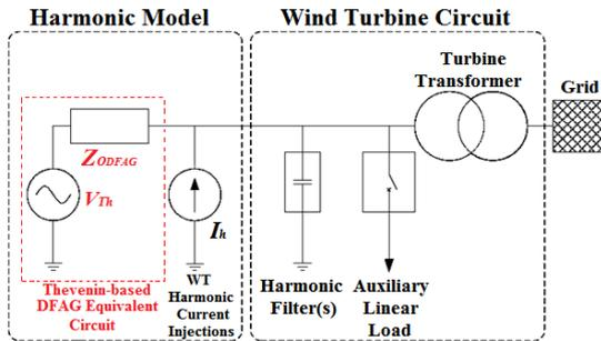
Fig. 1. Harmonic model of a DFAG based on [8, 13, 17, 30].
