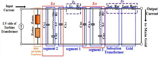
Fig. 7. Equivalent circuit of PE TF from WT1 to the grid.
