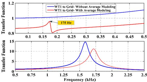
Fig. 10. PE TF from WT1 to the grid with and without converter average modelling. Upper figure: 0-0.5 kHz; lower figure: 0.5-2.5 kHz.
