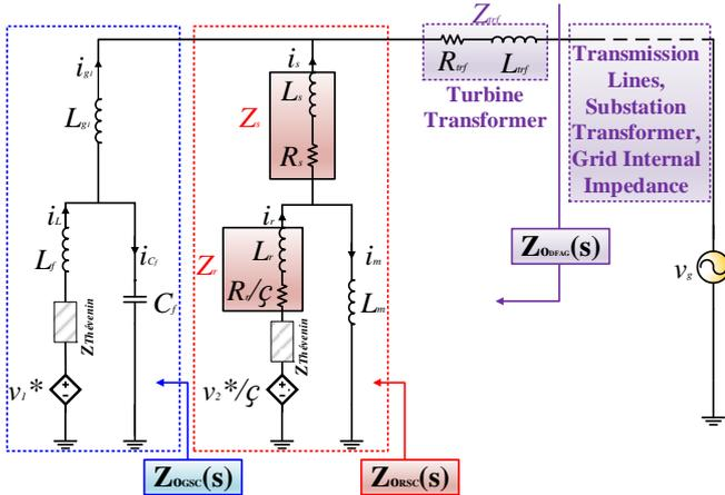
Fig. 5. Equivalent DFAG output impedance.
