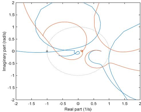
Figure 5 Nyquist curves used in the  $dq$ -impedance method (Gain margin: -5.76 dB at 157.34 Hz, Phase margin: -2.44° at 139.72 Hz).
