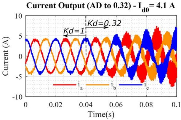
Figure 9 Experimental results of the VSC current output when  $K_d$  changed from 1 to 0.32.
