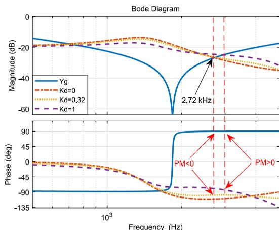
Figure 8 Impedance-based stability analysis with and without active damping in Bode diagram – grid impedance  $Y_g$  as solid blue line, VSC input admittance with  $K_d=0$  as dash-dotted orange line, with  $K_d=0.32$  as dotted yellow line, with  $K_d=1$  as dashed purple line.
