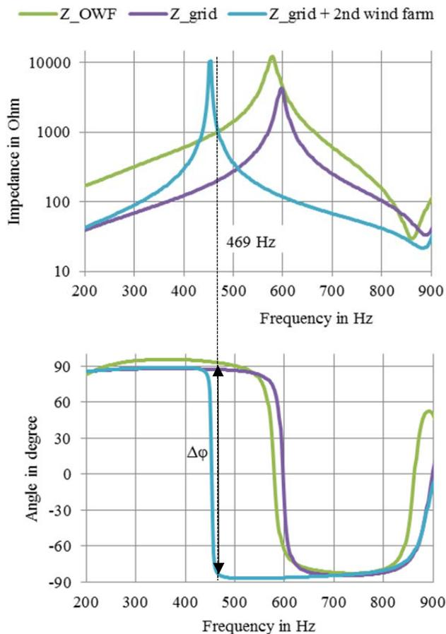
Figure 2 Impedance-based stability analysis of the offshore wind farm before and after energizing the second wind farm.
