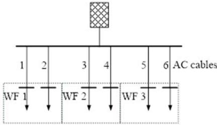
Figure 10 Example of several power electronics devices connected to a common point of connection.
