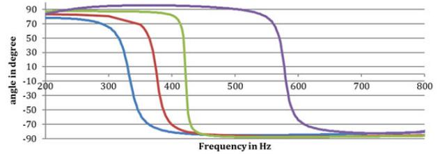
Figure 11 Frequency scans taken at cable 1 at the wind farm side for the impedance-based analysis
