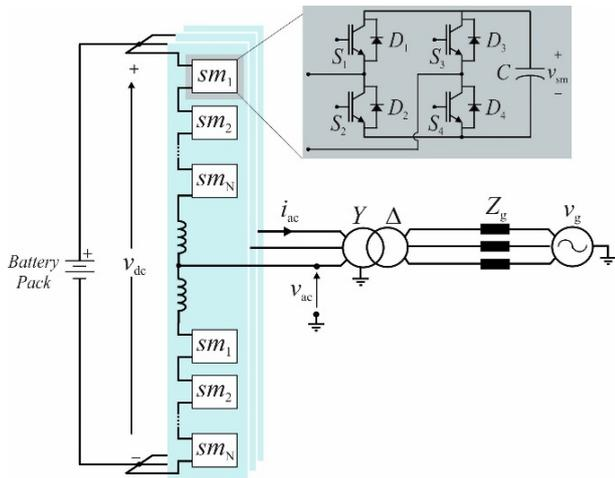
**Fig. 1. Double star full-bridge (DSFB) MMC with centralized energy storage (CES).**
