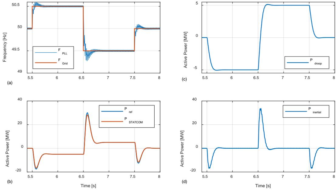
**Fig. 5. Frequency response by STATCOM with BESS: (a) Actual ( $F_{Grid}$ ) and measured ( $F_{PLL}$ ) grid frequency. (b) Active power injection- reference ( $P_{ref}$ ) and injected ( $P_{STATCOM}$ ). (c) Active power reference for frequency droop response. (d) Active power reference for inertial power reference.**
