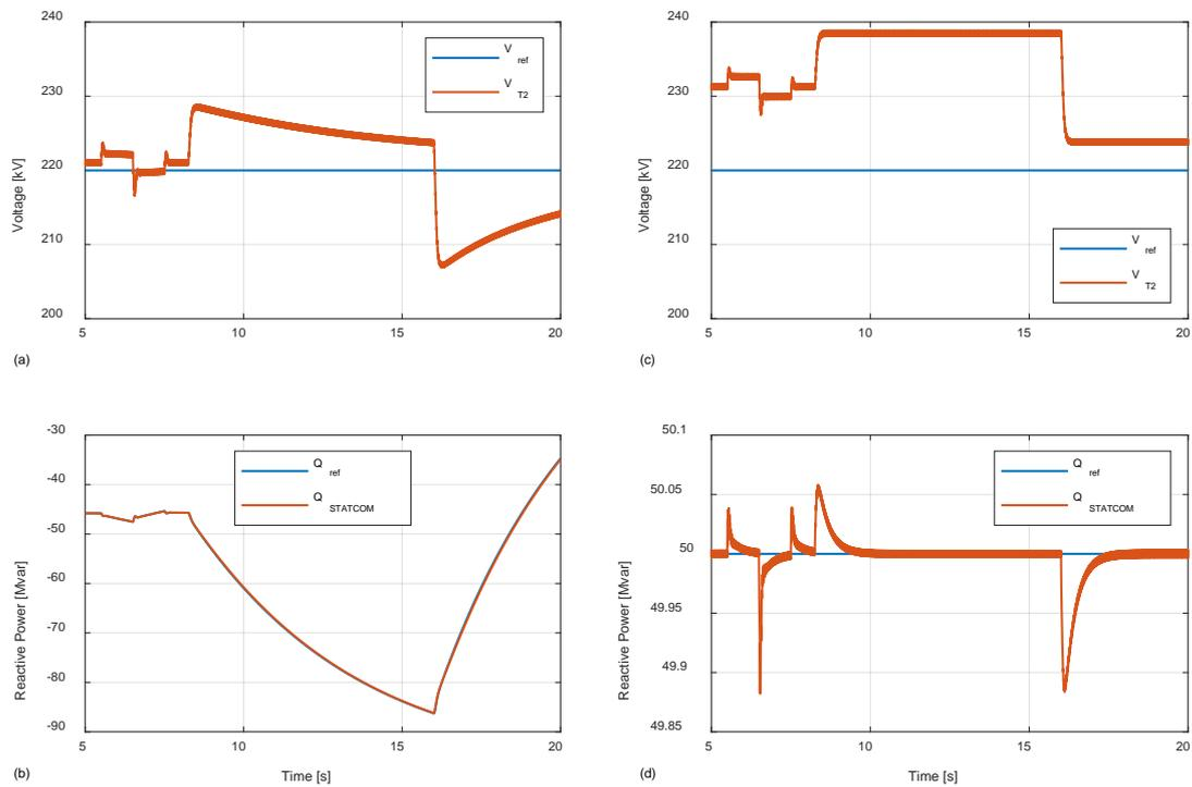
**Fig. 6. Voltage support by STATCOM: (a) Terminal voltage at T2 with voltage support from STATCOM. (b) Reactive power reference ( $Q_{ref}$ ) and injected reactive power from STATCOM for voltage support. (c) Terminal voltage at T2 without any voltage support from STATCOM. (d) Constant reactive power reference ( $Q_{ref}$ ) of 50 Mvar and injected reactive power from STATCOM.**
