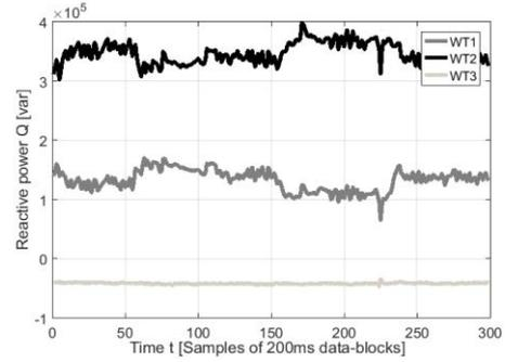
Fig. 5: The reactive power injection for all three WTs during 1 minute of operation, when PWM synchronizations feature is enabled and the active power operating point is approximately 30%.
