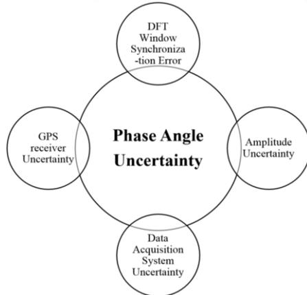
Fig. 4: The phase measurement uncertainty sources [14].
