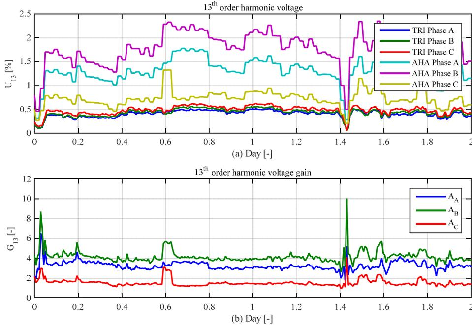
Figure 7 (a) Trige 400 kV and Anholt 33 kV harmonic 13<sup>th</sup> order voltages and (b) corresponding harmonic voltage gains.
