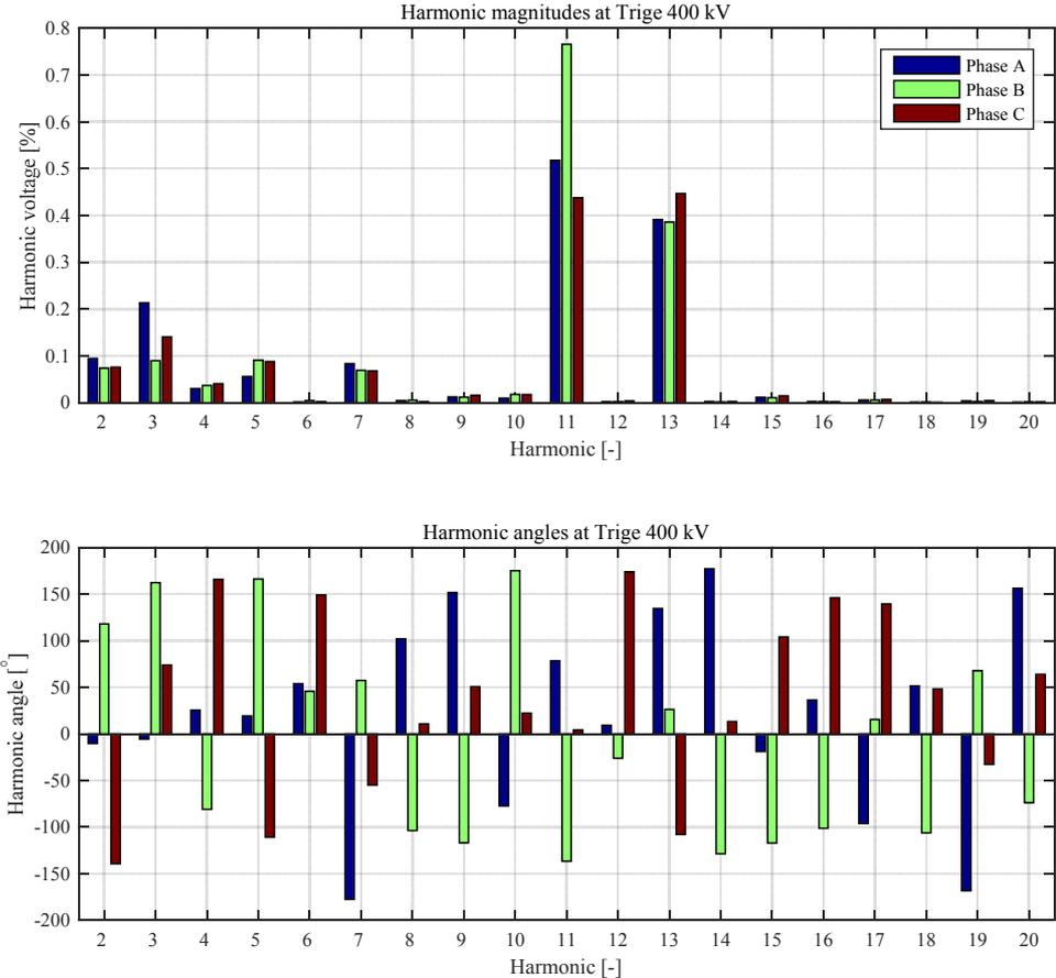
Figure 2 Harmonic magnitudes and phase angles obtained at Trige 400 kV.
