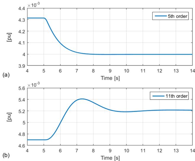
Fig. 13. Harmonic voltages at T1. (a) 5<sup>th</sup> order. (b) 11<sup>th</sup> order.
