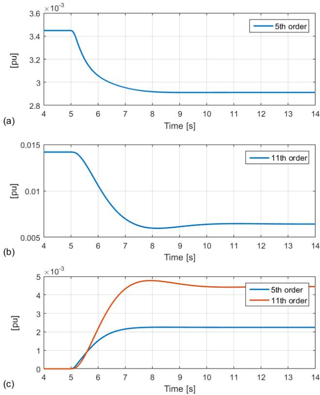
Fig. 12. (a) 5<sup>th</sup> harmonic voltage at T2. (b) 11<sup>th</sup> harmonic voltage at T2. (c) 5<sup>th</sup> and 11<sup>th</sup> harmonic resistive currents by the STATCOM.
