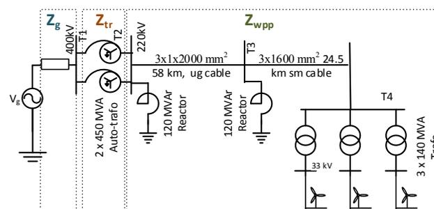
Fig. 1. WPP electrical network model.
