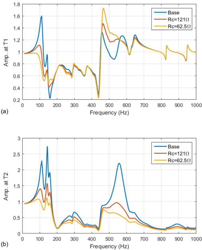
Fig. 8. Amplification due to compensation at T2.
