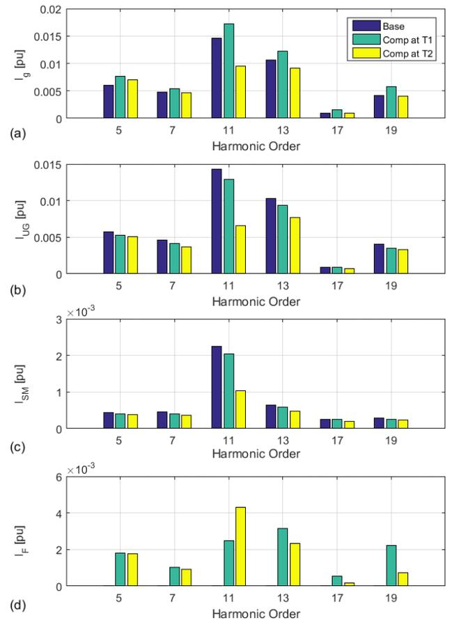
Fig. 11. Harmonic currents in pu. (a) Grid at T1. (b) Underground cable at T2. (c) Sub-marine cable at T4. (d) STATCOM.
