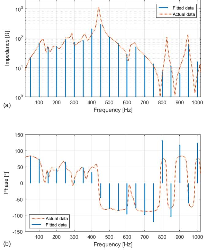
Fig. 3. Grid impedance characteristics. (a) Magnitude, and (b) Phase angle.
