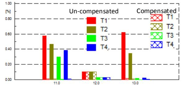
Fig. 7. Comparison of harmonic distortion in the un-compensated (solid bars) and the system with 11<sup>th</sup> and 13<sup>th</sup> harmonic current compensation (solid bars) at the bus T1.
