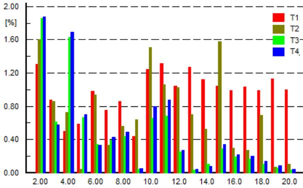
Fig. 5. Harmonic distortion at the bus T1, T2, T3 and T4 for 1% background harmonics in the grid.
