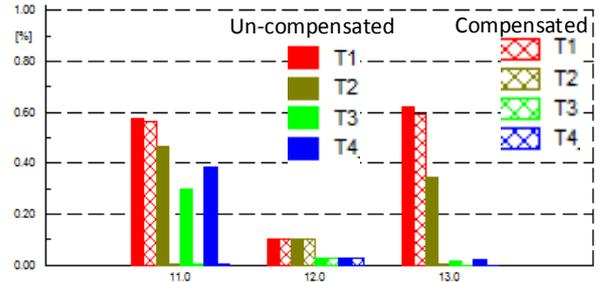
Fig. 8. Comparison of harmonic distortion in the un-compensated (solid bars) and the system with 11<sup>th</sup> and 13<sup>th</sup> harmonic current compensation (solid bars) at the bus T2.
