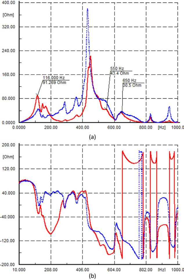
Fig. 3. Positive and negative sequences (thick, red) and zero sequence (dotted, blue) components of the transfer impedance between bus T1 and T2 (a) Magnitude. (b) Phase.
