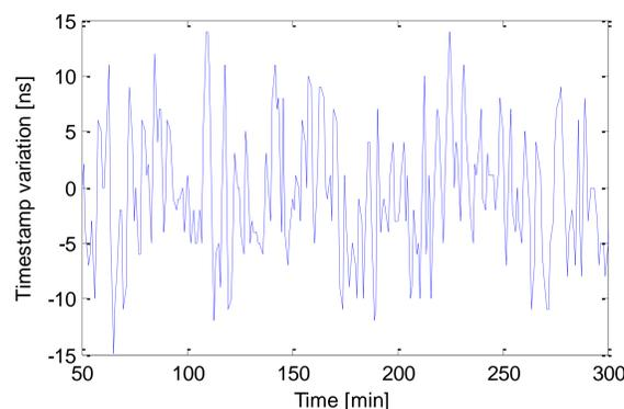
Figure 2 Variation of pulse-per-second signal synchronized with a GPS timestamp using phase-locked loop
